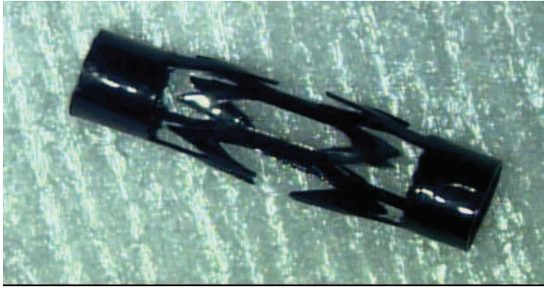
Figure 2.6 Final fabricated and crosslinked stent
